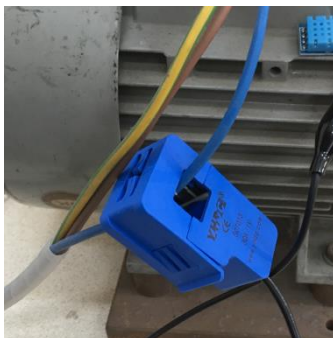
Figure 5. Current sensor of proposed data acquisition system
