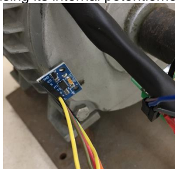
Figure 4. Vibration sensor of proposed data acquisition system
